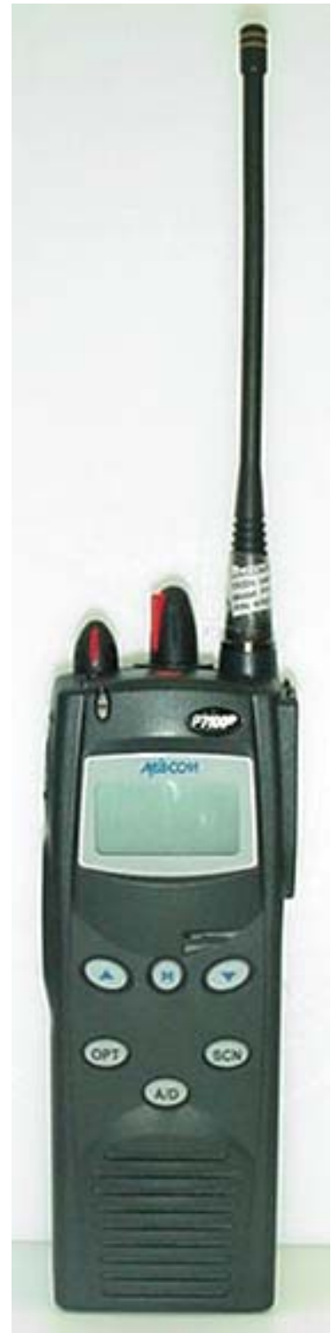
Front of DUT (S/N: T1PA-UL03) P/N: RU101219V61 R1B (Scan) with Quarter-Wave Whip Antenna (P/N: KRE1011223/10)
