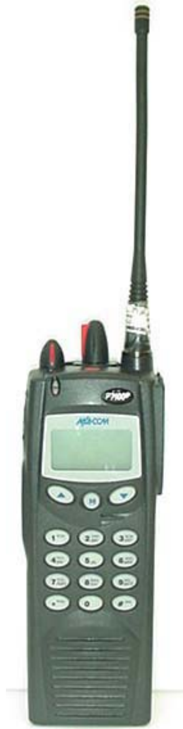
Front of DUT (S/N: T1PA-UL10) P/N: RU101219V62 R1B (System) with Quarter-Wave Whip Antenna (P/N: KRE1011223/10)
