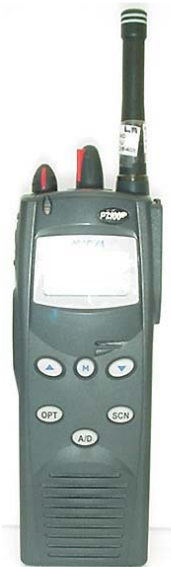
Front of DUT (S/N: T1PA-UL03) P/N: RU101219V61 R1B (Scan) with Helical Coil Antenna (P/N: KRE1011219/9)
