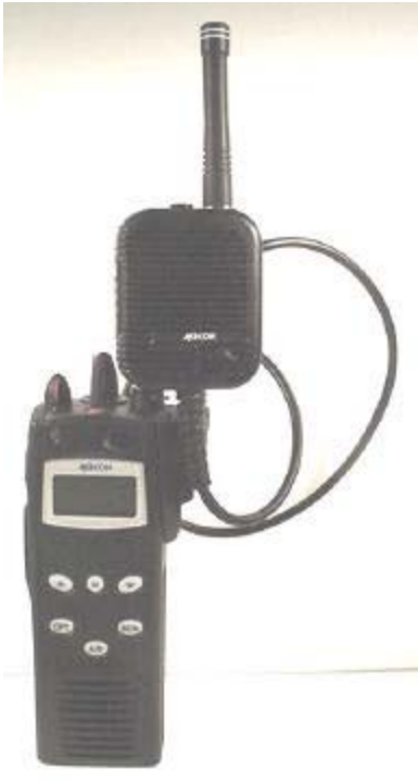
with Speaker-Mic Antenna Version Plus (P/N: KRY1011617/184R1A) Helical Coil Antenna (P/N: KRE1011219/9)
