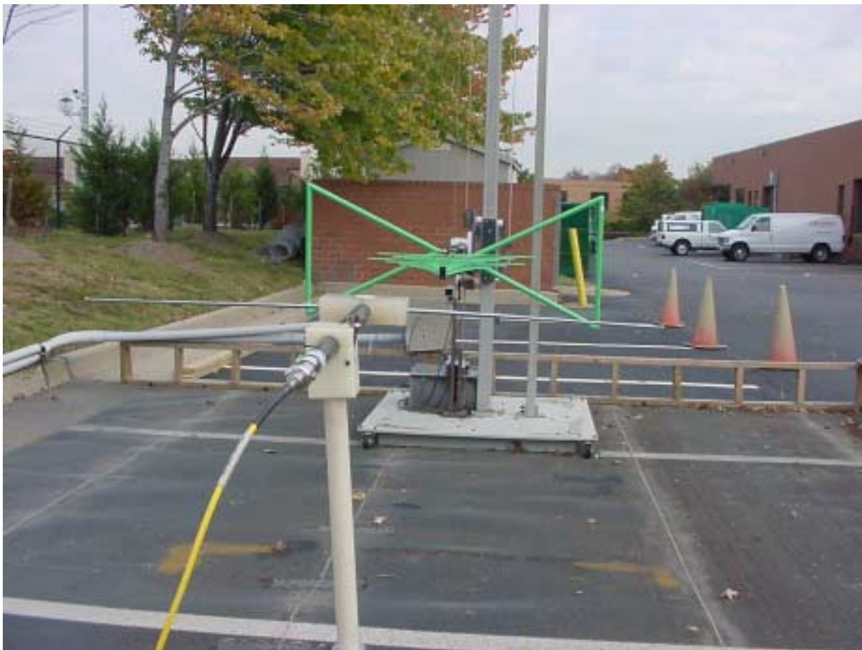
PHOTOGRAPH 3: SUBSTITUTION TRANSMITTING DIPOLE ANTENNA USED FOR FREQUENCIES (30 MHZ – 1 GHZ)
