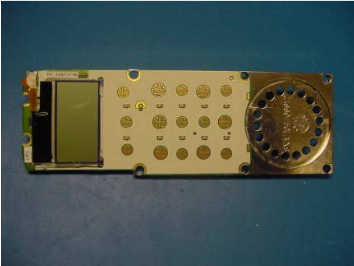
PHOTOGRAPH 18: FRONT OF SECONDARY PCB WITH LCD
