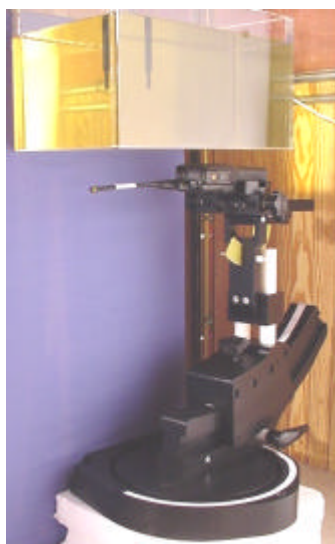
Face-held SAR Test Setup with small planar phantom
