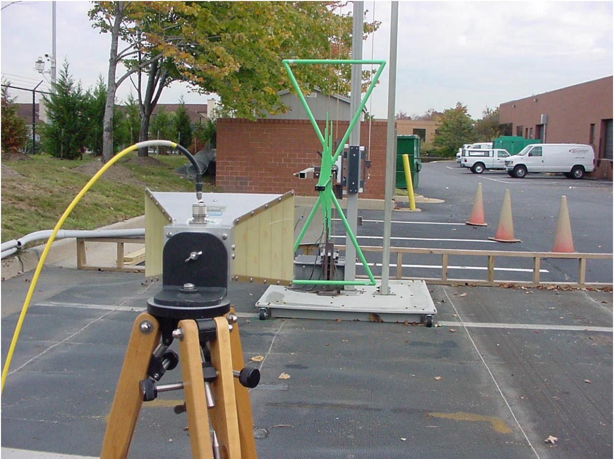
PHOTOGRAPH 4: SUBSTITUTION TRANSMITTING HORN ANTENNA USED FOR FREQUENCIES (1 GHZ-18 GHZ)
