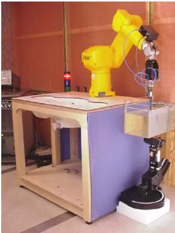
DASY3 SAR Measurement System with small planar phantom
