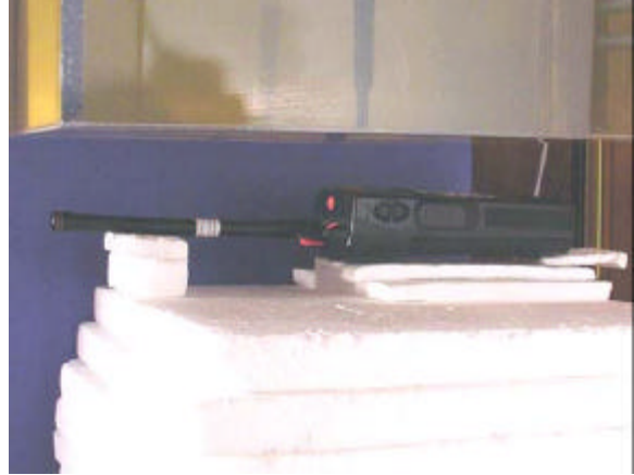
2.5cm Separation Distance - Antenna #1 (136-151MHz)
