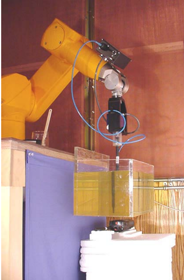
2.5cm Separation Distance - Antenna #1 (136-151MHz)
