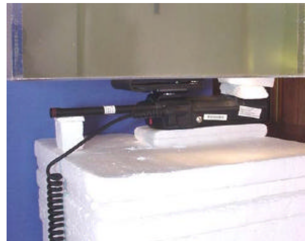
3.5cm Belt-Loop Separation - Antenna #3 (162-174MHz)
