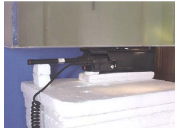
1.7cm Case/Loop Separation - Antenna #3 (162-174MHz)
