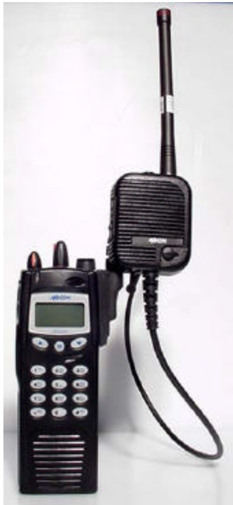
Front of EUT with Speaker-Mic Antenna Version Plus (P/N: KRY1011617/84R1A, KRY1011617/184R1A) & Antenna #2 (P/N: KRE1011219/2)
