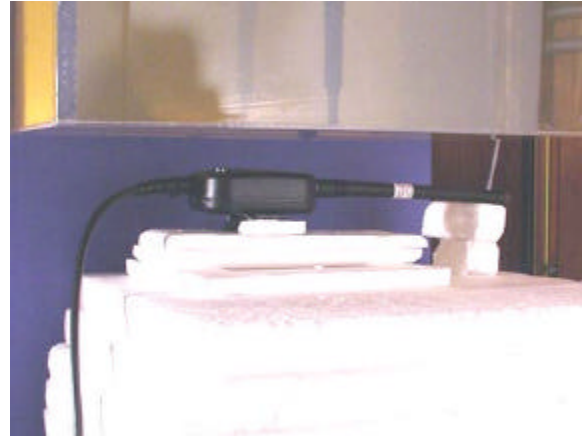
2.5cm Separation Distance - Antenna #1 (136-151MHz)
