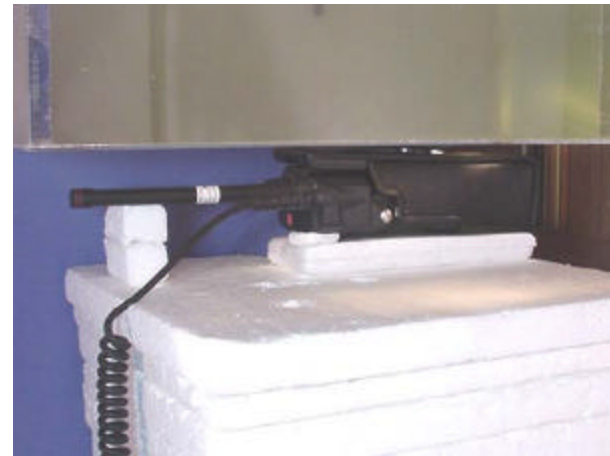
1.7cm Case/Loop Separation - Antenna #2 (150-162MHz)
