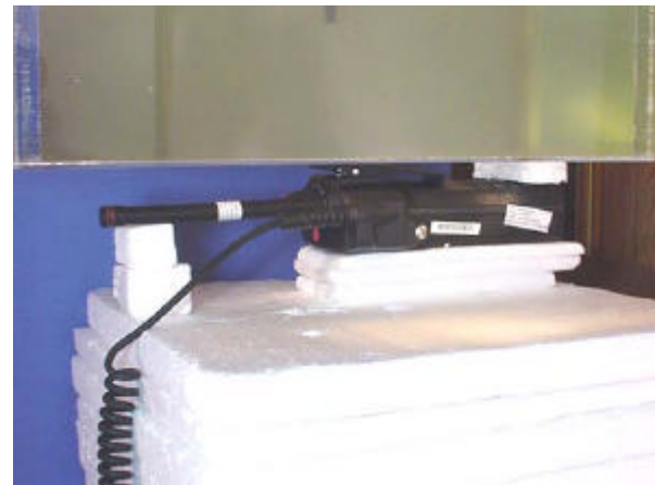
1.1cm Belt-Clip Separation - Antenna #3 (162-174MHz)
