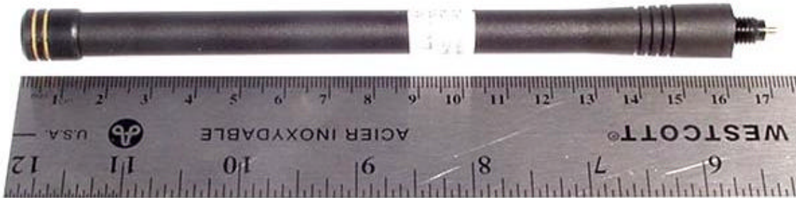
Helical Coil Antenna #1 - 136-151MHz (P/N: KRE1011219/1)
