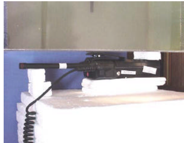
1.1cm Belt-Clip Separation - Antenna #2 (150-162MHz)
