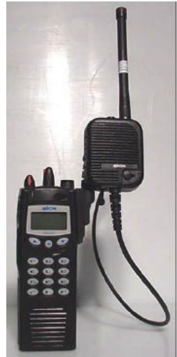
Front of EUT with Speaker-Mic Antenna Version Plus (P/N: KRY1011617/84R1A, KRY1011617/184R1A) & Antenna #3 (P/N: KRE1011219/3)
