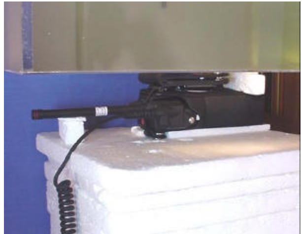
4.0cm Case & Loop Separation - Antenna #2 (150-162MHz)
