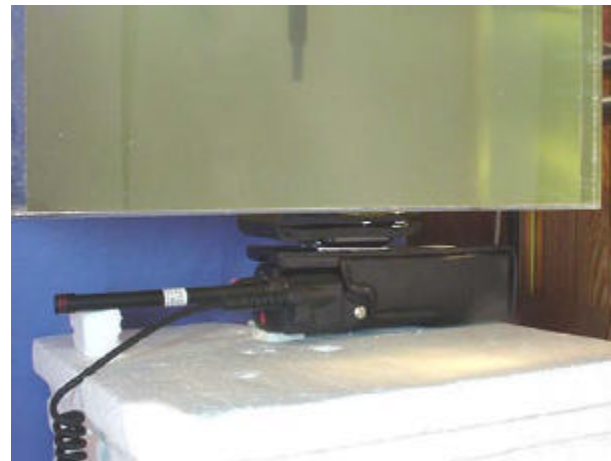
4.5cm Case & Loop Separation - Antenna #2 (150-162MHz)
