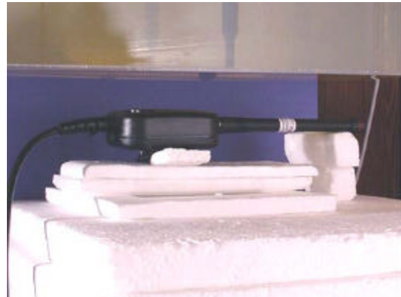
2.5cm Separation Distance - Antenna #3 (162-174MHz)
