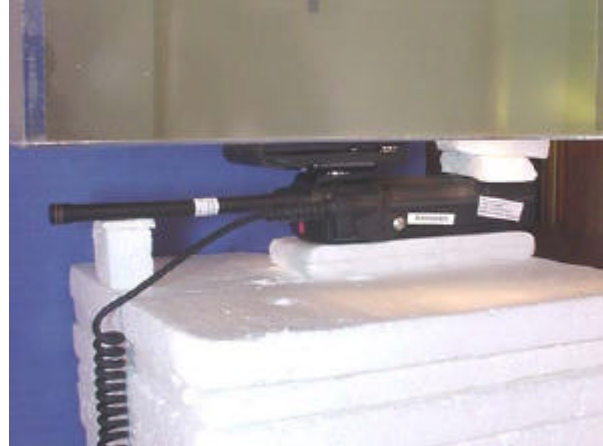
3.5cm Belt-Loop Separation - Antenna #1 (136-151MHz)
