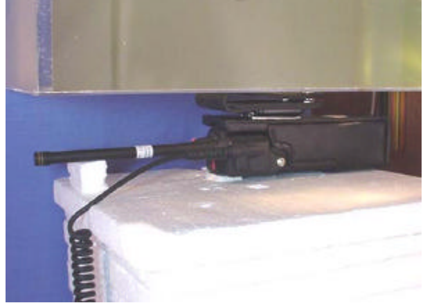
4.5cm Case & Loop Separation - Antenna #1 (136-151MHz)
