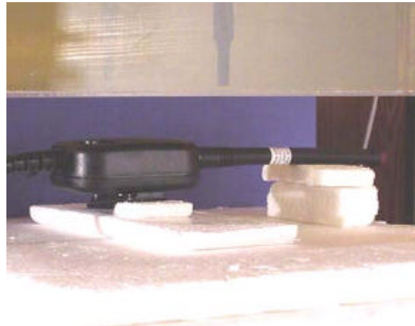
2.5cm Separation Distance - Antenna #2 (150-162MHz)
