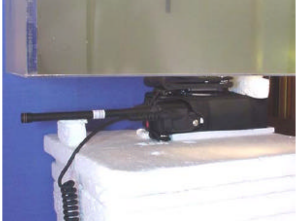
4.0cm Case & Loop Separation - Antenna #1 (136-151MHz)
