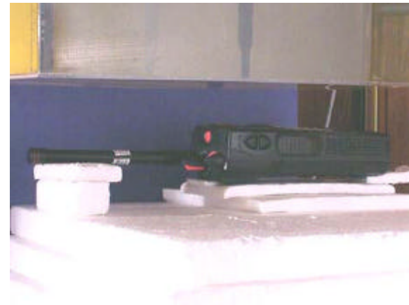
2.5cm Separation Distance - Antenna #3 (162-174MHz)
