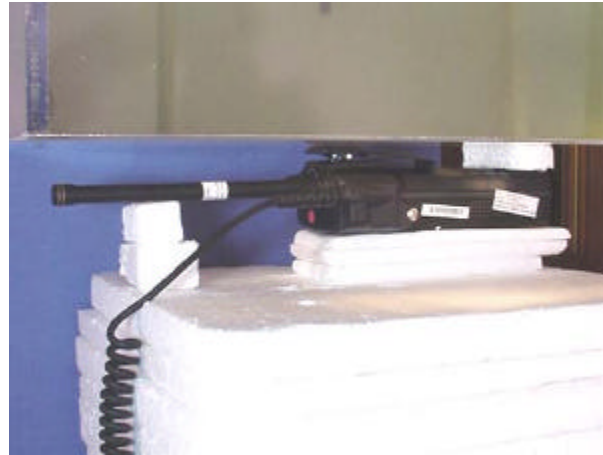
1.1cm Belt-Clip Separation - Antenna #1 (136-151MHz)
