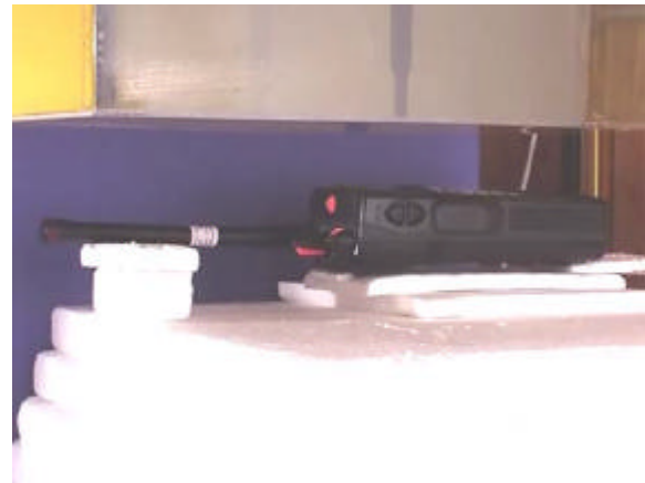
2.5cm Separation Distance - Antenna #2 (150-162MHz)
