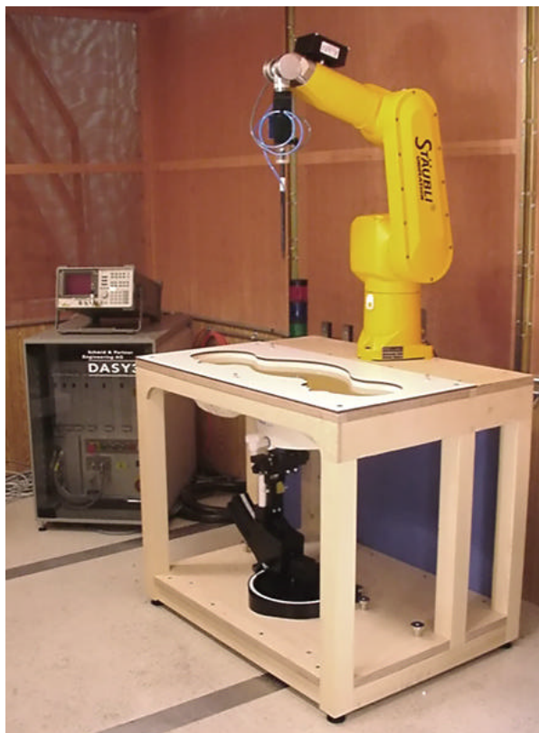
DASY3 SAR Measurement System with SAM phantom
