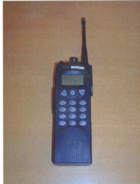
(b) The Ericsson Jaguar 700P with \lambda/4 antenna (configuration 2).
