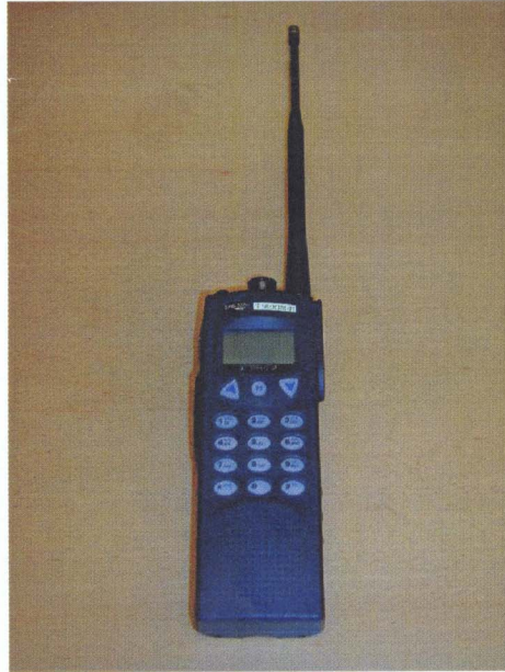
(a) The Ericsson Jaguar 700P with \lambda/2 antenna (configuration 1).
