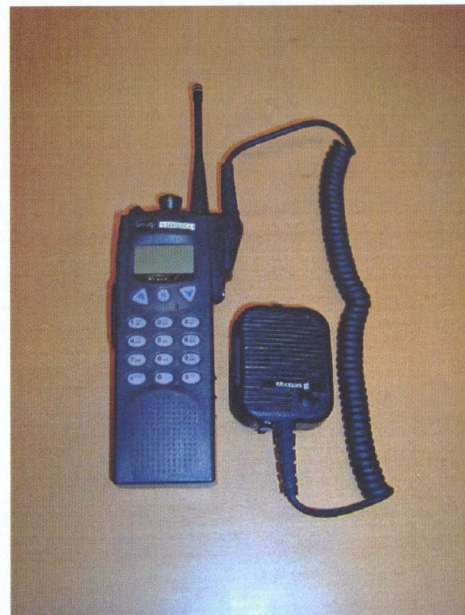
(d) The Ericsson Jaguar 700P with \lambda/4 , beltclip and speaker/microphone (configuration 4).
