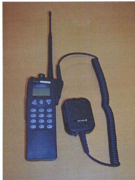
(c) The Ericsson Jaguar 700P with \lambda/2 , beltclip and speaker/microphone (configuration 3).
