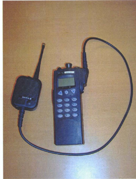
(f) The Ericsson Jaguar 700P with beltclip and \lambda/4 antenna mounted on the speaker/microphone (configuration 6).
