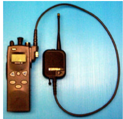
Left: Jaguar 700P with \lambda/2 antenna, speaker/microphone, and belt clip – back showing belt clip
