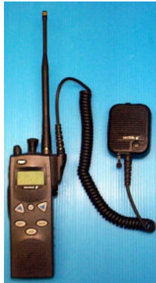
Left: Jaguar 700P with \lambda/2 antenna, speaker/microphone, and belt clip – back showing belt clip
