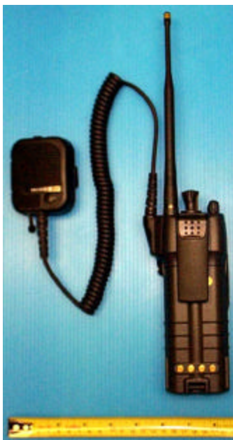
Left: Jaguar 700P with \lambda/2 antenna, speaker/microphone, and belt clip – back showing belt clip
