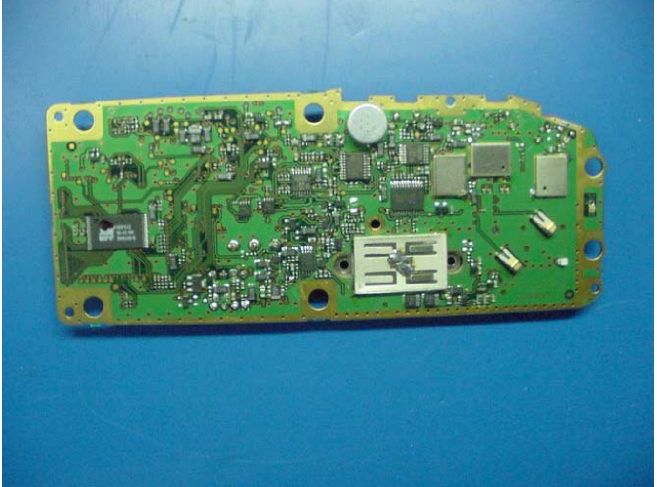
PHOTOGRAPH 9: MAIN PCB WITH SHIELDS FRONT SIDE
