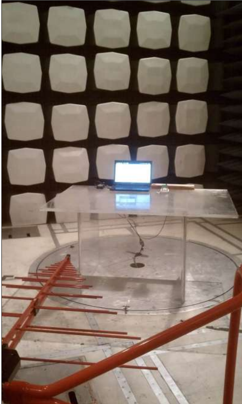
Photograph 1. Radiated Emissions, Test Setup
