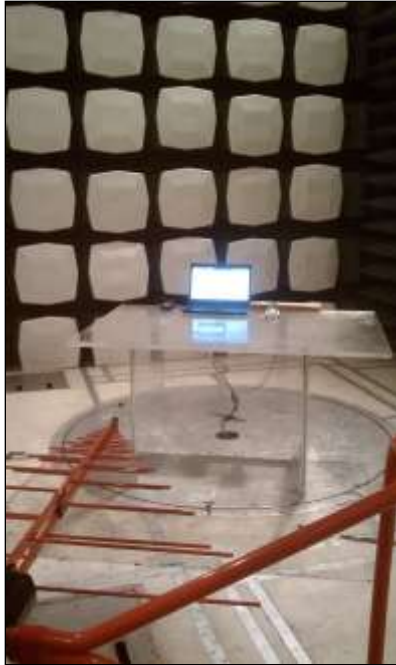
Photograph 2. Radiated Spurious Emissions, Test Setup
