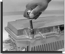
Step 1 – Loosen the 5/16 - 18 bolts holding the housing cover to base to open the housing cover.
