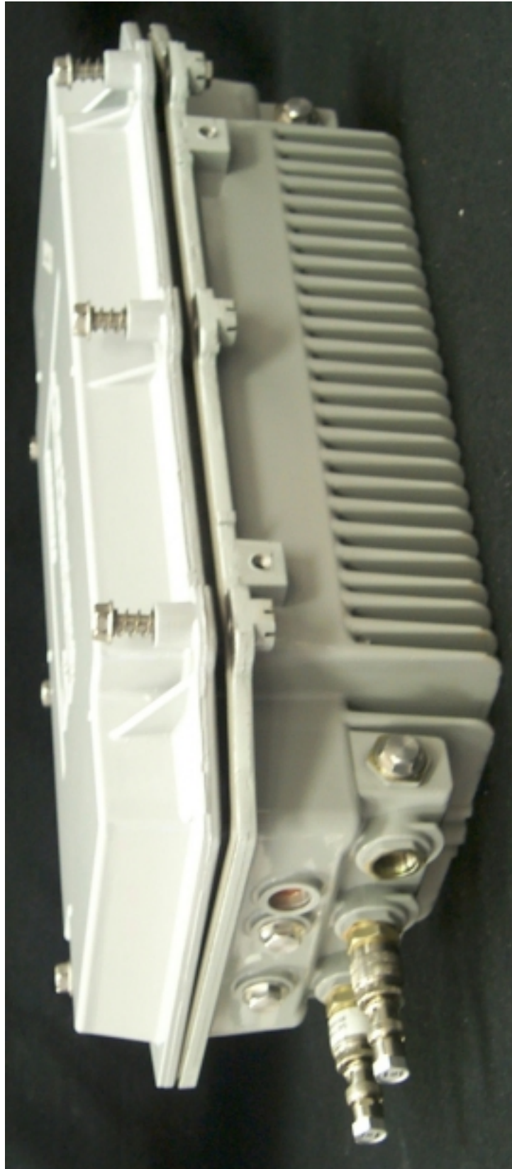
Photo 1. Front View of RF Network Amplifier
