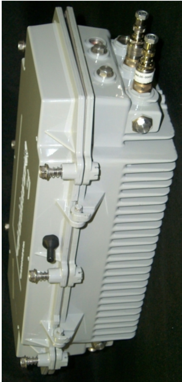
Photo 2. Rear View of RF Network Amplifier, Showing Mounted Antenna
