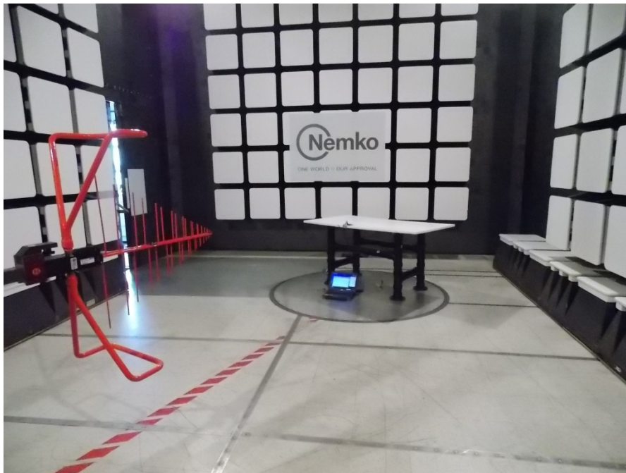
Figure 8.4-2: Spurious emissions (except for harmonics) setup photo
