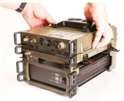
6. Fold the side latches back into position and turn the fasteners to secure.
