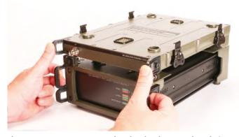
4. To secure the SDS, [rst rotate the lock clamps back into a vertical position, then turn the fasteners a quarter turn. The locks should click into place.
