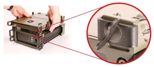
3. Push the SDS towards the rear of the power supply as shown below so that the capstans and SDS click into place.
