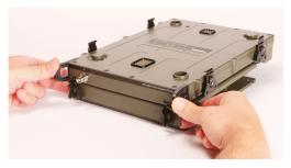
3. To secure the SDS, first ensure that the lock clamps are connected to the slots on the front of the SDS, then turn the fasteners a quarter turn.
