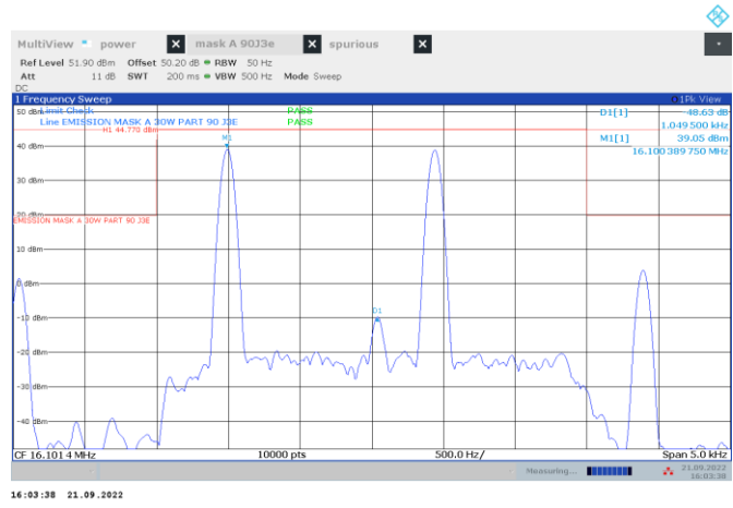
Figure 8.4-2: Mid channel 30W 400 Hz and 1800 Hz 40 dB Carrier suppression
