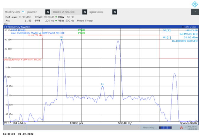
Figure 8.3-8: Mid channel 30W 400 Hz and 1800 Hz 40 dB Carrier suppression
