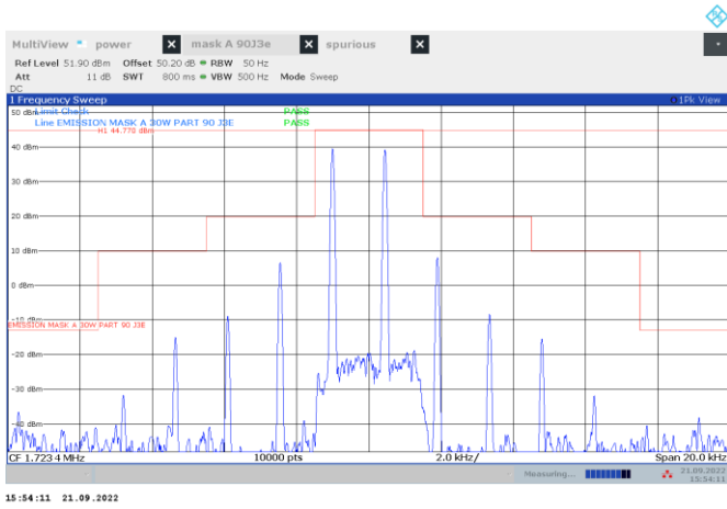
Figure 8.3-1: Low channel Mask 30W 400 Hz and 1800 Hz
