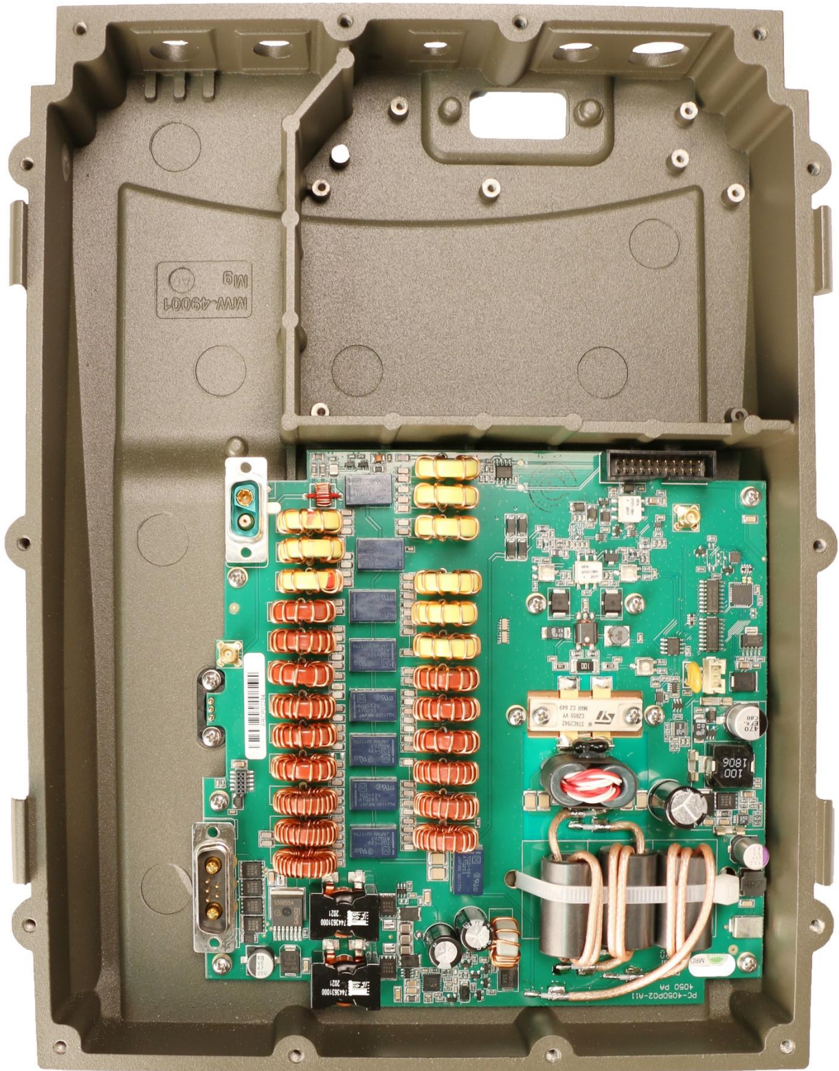
PRC-4090 Transceiver - PA board in chassis
