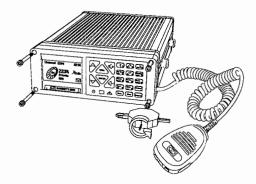
Remove the M4 cap screws from front panel using Barrett tool provided
