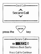
enter the station ID of the station you wish to call (see "Entering station ID's and using the address and telephone books") Note:- to make a secure call to multiple stations use a group call ID encompassing the required stations.
