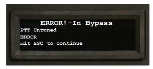
This error condition remains until the transceiver stops activating the amplifier's PTT line, and then clears automatically when the PTT is released.
