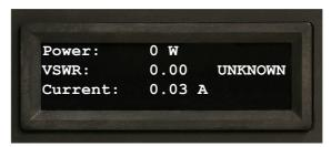
In this state the Linear will not operate when the transceiver begins to transmit. It will signal a fault to the 4050 transceiver and it will keep the Linear in bypass mode in order to protect whatever is connected and it will display the error message.
