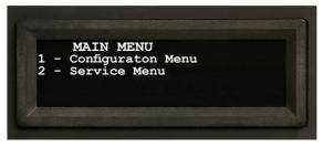
Use the navigation keys to select the desired menu and then press the ENT key.
