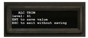
Use the UP and DOWN navigational keys to change the value which ranges from 0 to 63. Press ENT to save the new value or ESC to exit without changing the setting value.
