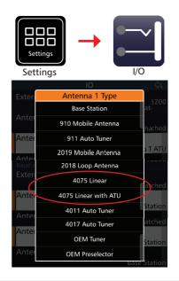
If '4075 not detected' appears on the transceiver display (see right) ensure that the following are not responsible before contacting Barrett Communications:
