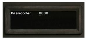
Use the UP and DOWN navigational keys to select the digit value and the LEFT and RIGHT navigational keys to select the digit being set. Once done, press ENT and the following warning will display:
