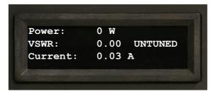
As with the 'Unknown Tuner' and 'Missing Tuner' modes, if the 4050 Transceiver attempts to operate the amplifier when 'Untuned', the amplifier signals a fault to the 4050, displays the following screen and engages the bypass mode so that the RF output of the 4050 is not amplified in order to protect the attached tuner.
