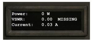
As with the Unknown Tuner, if the 4050 transceiver attempts to activate the amplifier with a Missing Tuner, a fault is generated.
