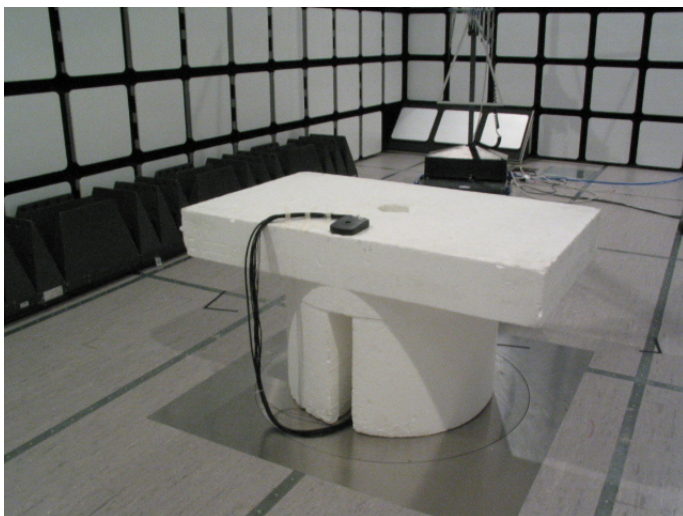
Picture 2 Radiated emission measurement Bluetooth TX
