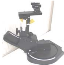
Device holder supplied by SPEAG
