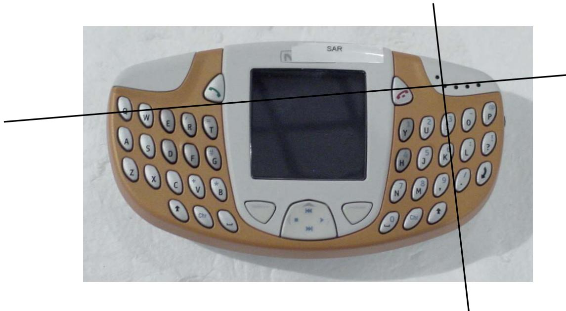
**The reference lines are shown in the photo above. Positioning is based on the asymmetric design of the phone and location of the earpiece.**
