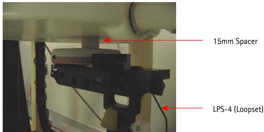
Note: the 15mm spacer was removed before the SAR measurement.
