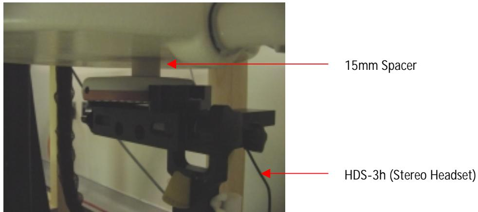
Note: the 15mm spacer was removed during the SAR measurement.
