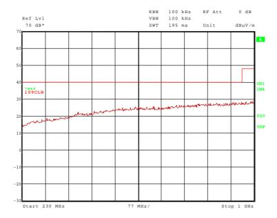
No significant frequencies at least 13 dB below the limit found. Therefore no final measurements on the open area test site were carried out.
