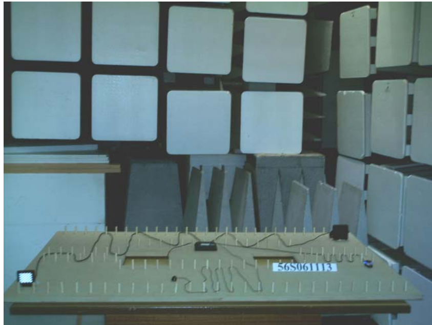
Radiated Emissions Test Setup (Front View)
