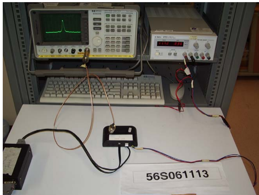
Spectrum Bandwidth (20dB Bandwidth Measurement) Test Setup
