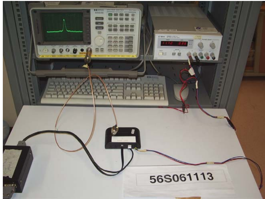
Carrier Frequency Separation Test Setup
