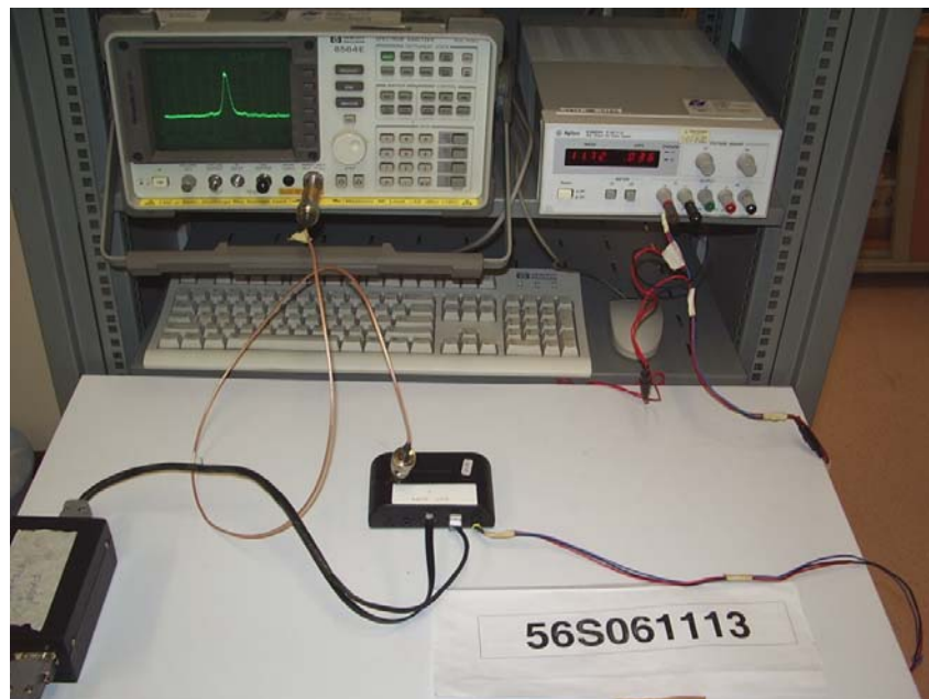
Average Frequency Dwell Time Test Setup
