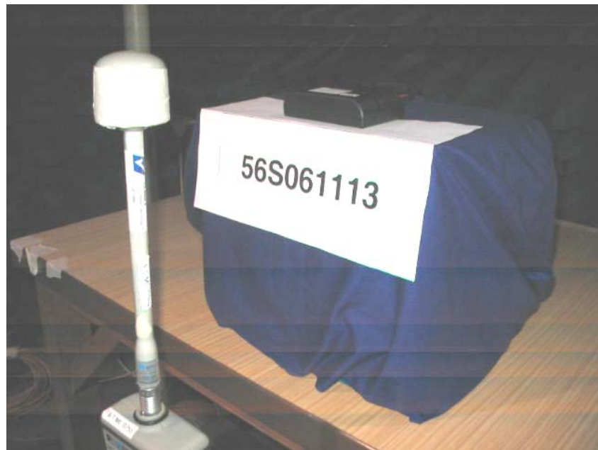
Maximum Permissible Exposure (MPE) Test Setup
