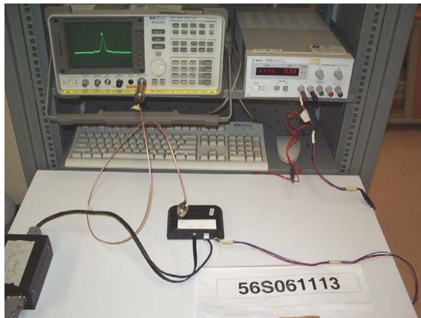
RF Conducted Spurious Emissions Test Setup
