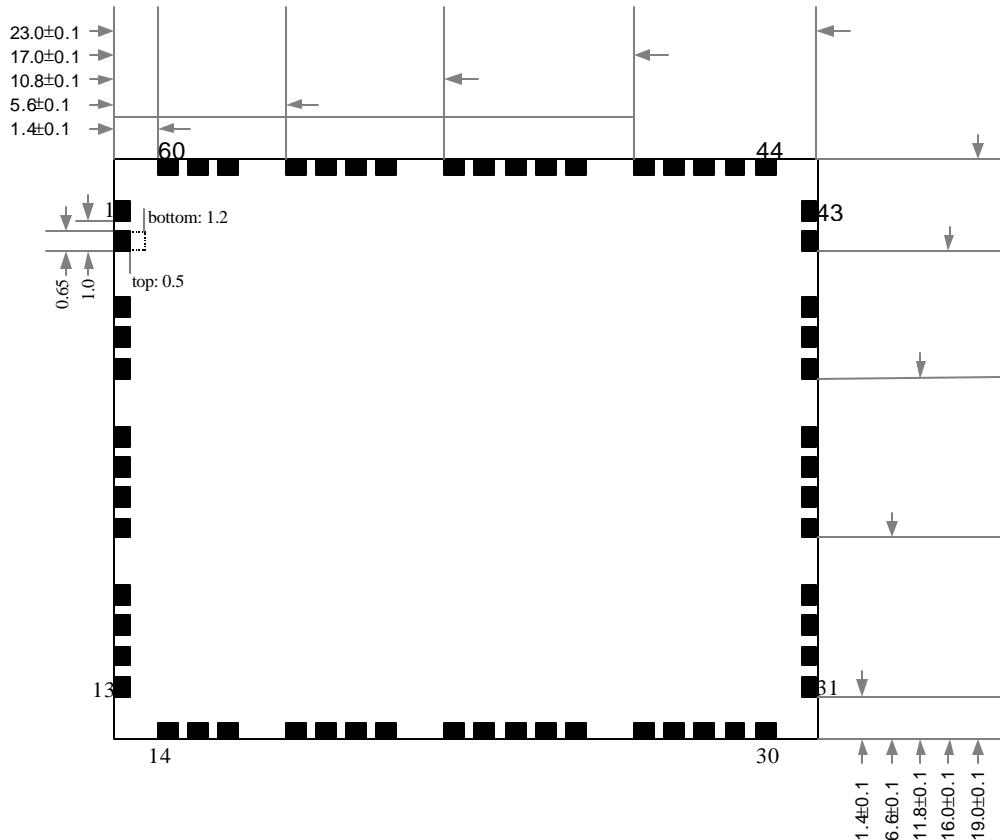
The figure on the right shows the detailed module pad dimensions. The pads include 400  $\mu\text{m}$  half-vias in order to achieve proper solderability on the edge of the PCB. The total height of the MCM including shielding is **2.0mm+/-0.1**. It is the sum of PCB-height (0.5mm), soldering gap (0.05mm) and assembled shielding components lid + frame (1.45mm).
