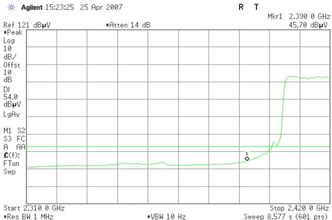
**Band Edges (IEEE 802.11g / CH High)****Detector mode: Peak****Polarity: Vertical**
