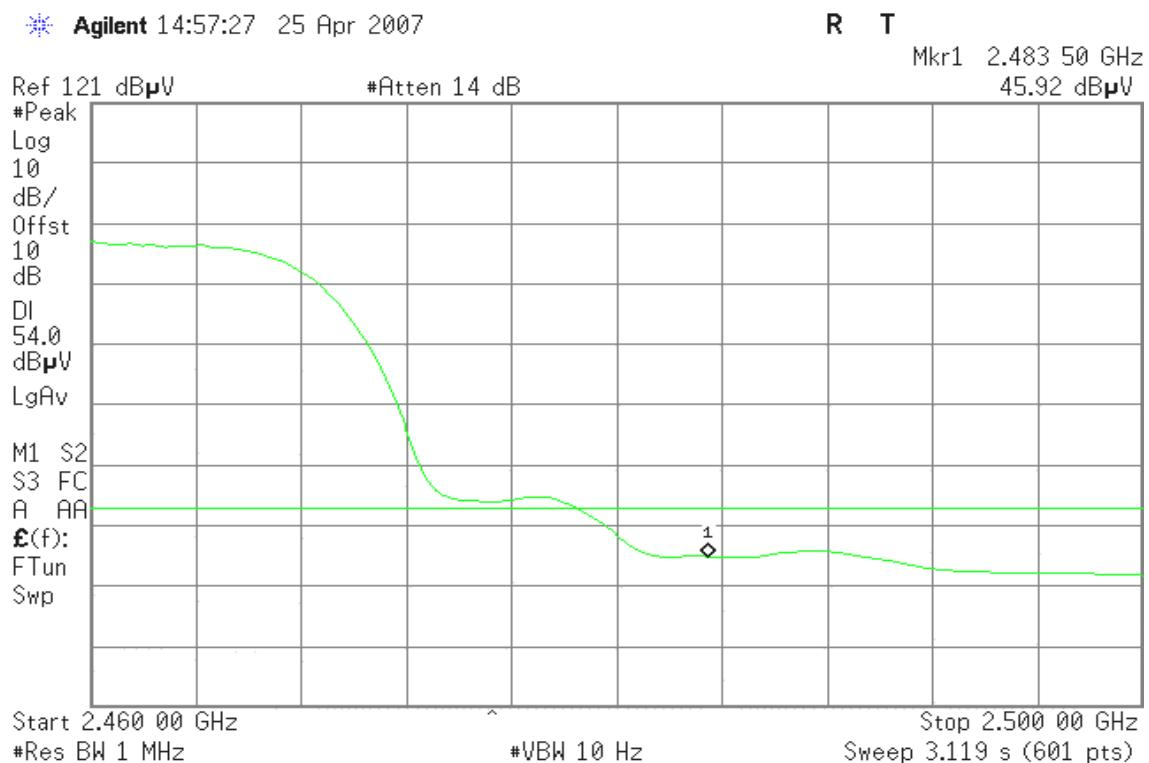
**Band Edges (IEEE 802.11g / CH Low)****Detector mode: Peak****Polarity: Vertical**
