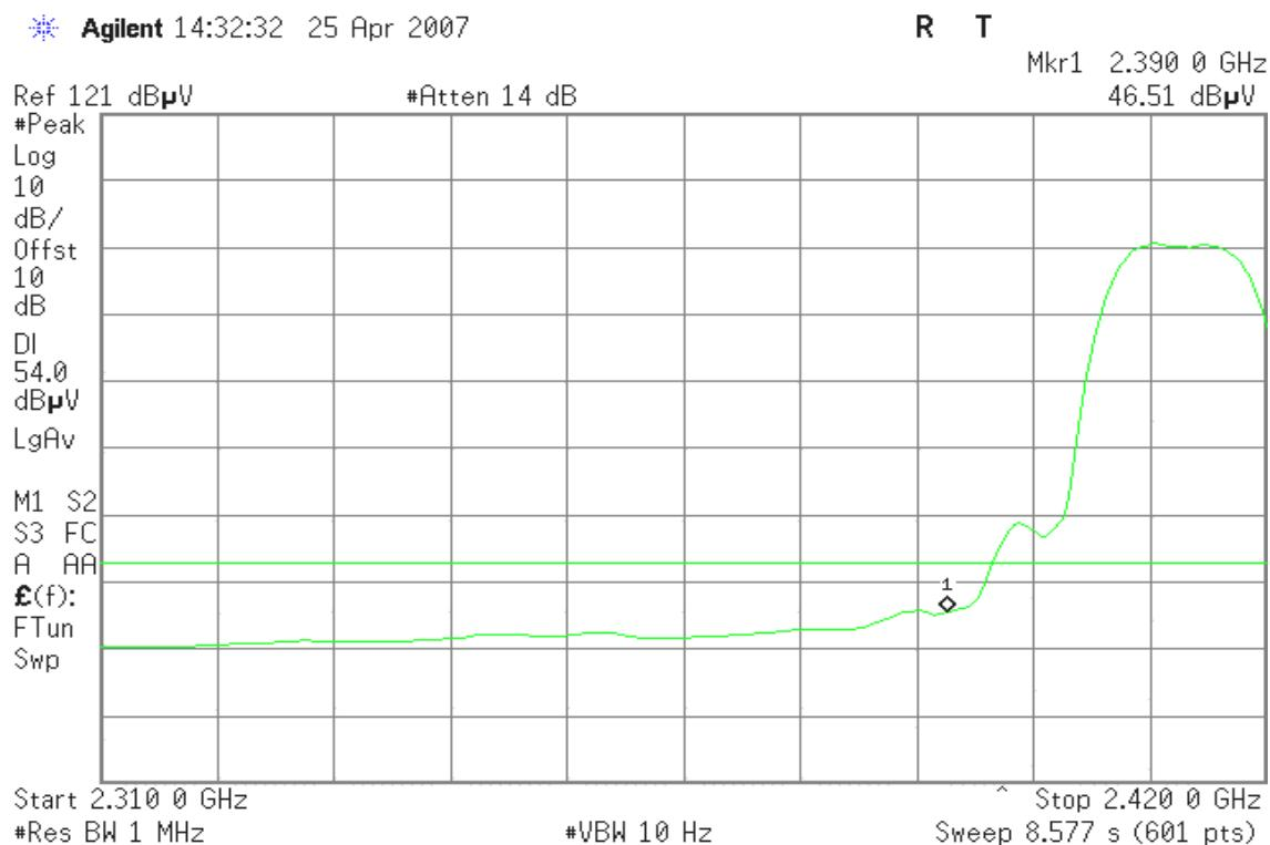
**Band Edges (IEEE 802.11b / CH High)****Detector mode: Peak****Polarity: Vertical**
