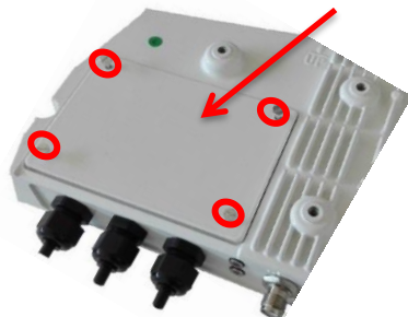
Cable glands (Data Bus-Power sup. - Input/Output)
