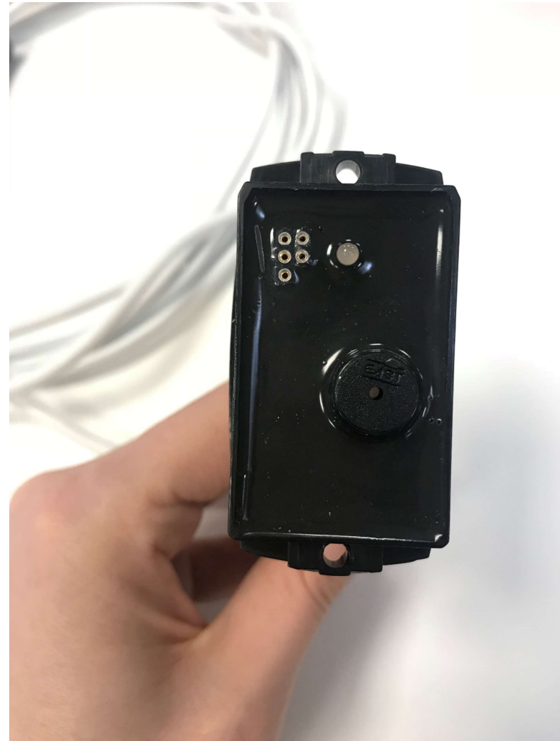
Motherboard integrated in the plastics after resin coating
