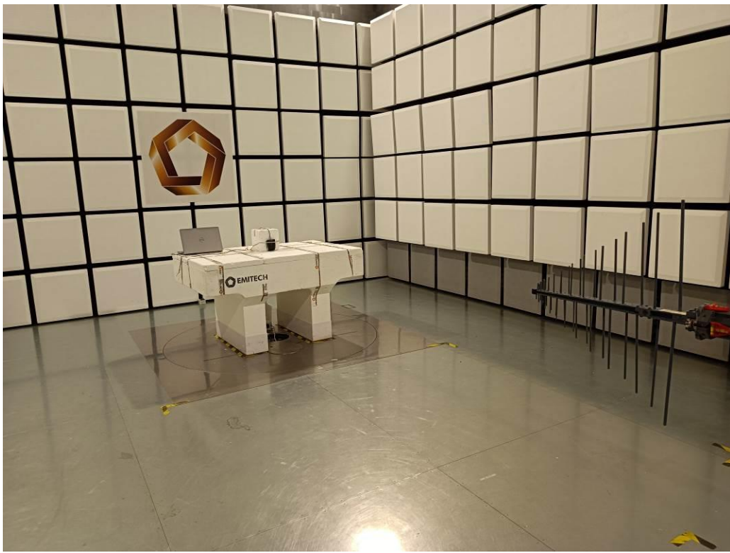
TEST SETUP PHOTO(S) - FOR 200MHZ < FREQ < 1GHZ
