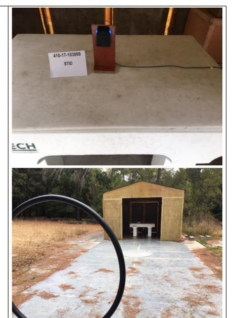
Measurement on open area test site (f<30MHz)
