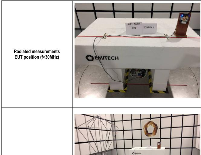
Radiated measurements (f>30MHz)
