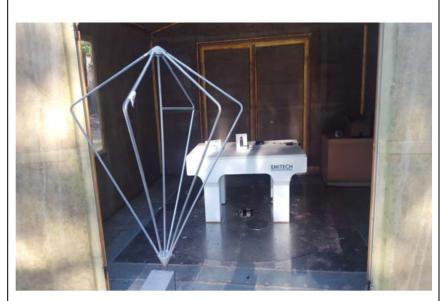
Radiated measurement on open area test site
