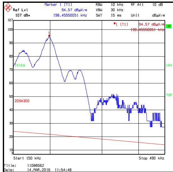
150 kHz to 490 kHz / average detector / EUT operating / measured at 300 metres on an open field test site
