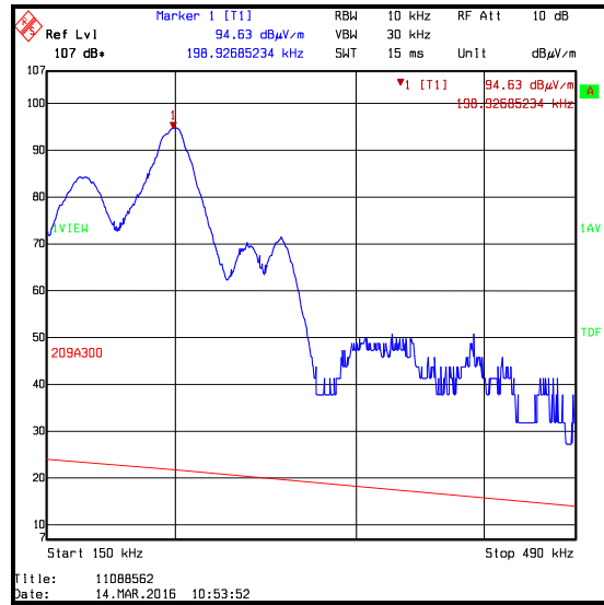
Frequency range: 150 kHz to 490 kHz Average detector / background scan
