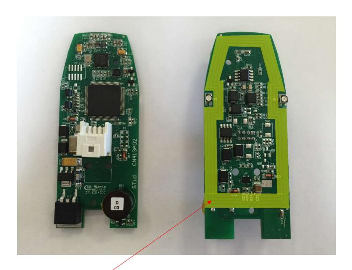
Loop antenna, directly printed on to the PCB
