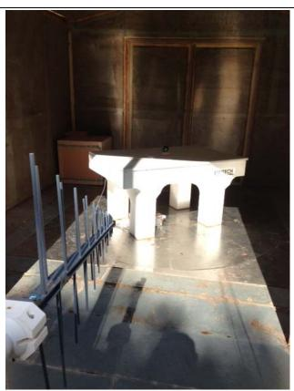
Radiated measurement on open area test site
