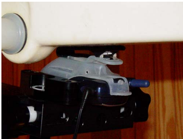
Figure 11.10 body SAR set-up (with holster, slide closed, antenna retracted position)
