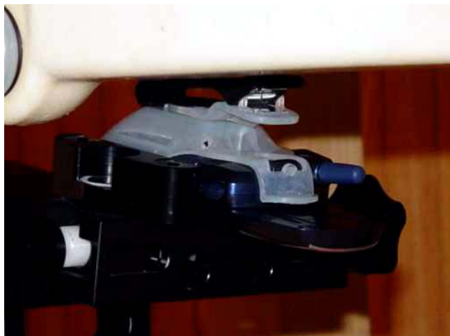
Figure 11.12 body SAR set-up (with holster, slide opened, antenna retracted position)
