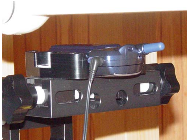
Figure 11.6 body SAR set-up (with 25.0mm air separation, slide closed, antenna retracted position)
