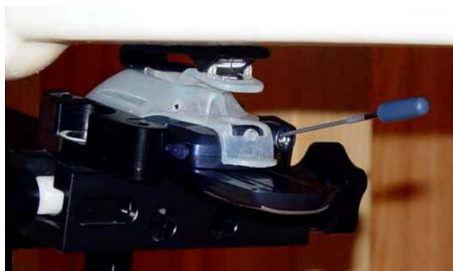
Figure 11.13 body SAR set-up (with holster, slide opened, antenna extended position)
