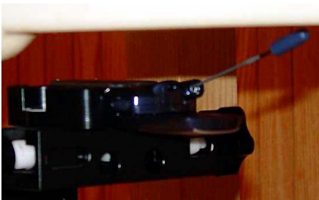
Figure 11.9 body SAR set-up (with 25.0mm air separation, slide opened, antenna extended position)
