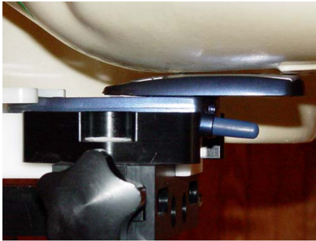
Figure 11.2 phone against the head (left cheek, slide opened, antenna retracted position)
