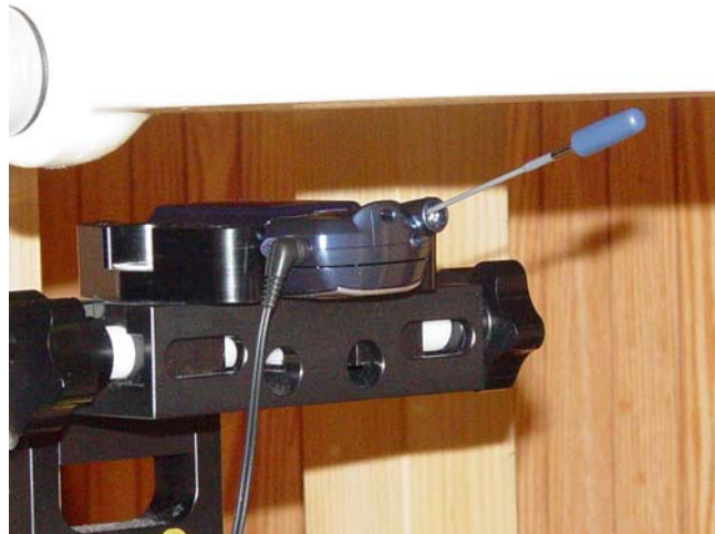
Figure 11.7 body SAR set-up (with 25.0mm air separation, slide closed, antenna extended position)
