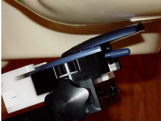
Figure 11.4 phone against the head (left tilt, slide opened, antenna retracted position)
