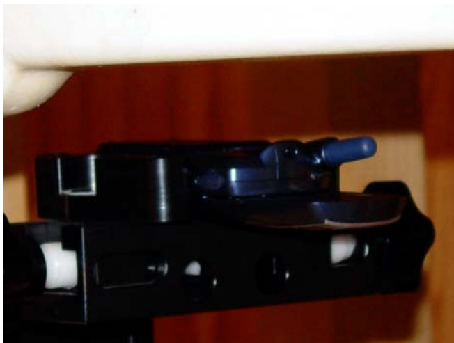
Figure 11.8 body SAR set-up (with 25.0mm air separation, slide opened, antenna retracted position)
