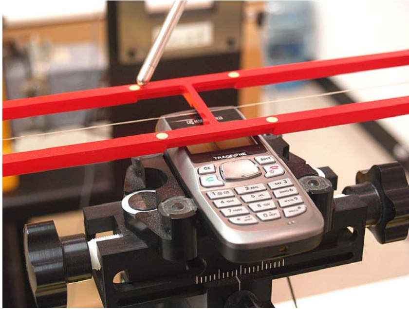
Figure 2 – HAC T-coil Test Setup
