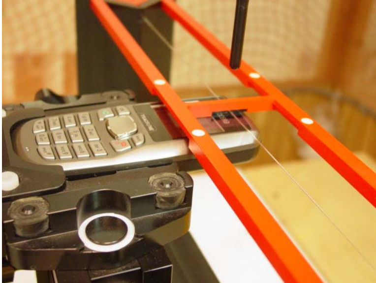
Figure 1b – HAC RF Emission Test Setup
