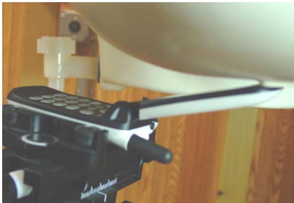
Figure 12.3 phone against the head (left tilt position)
