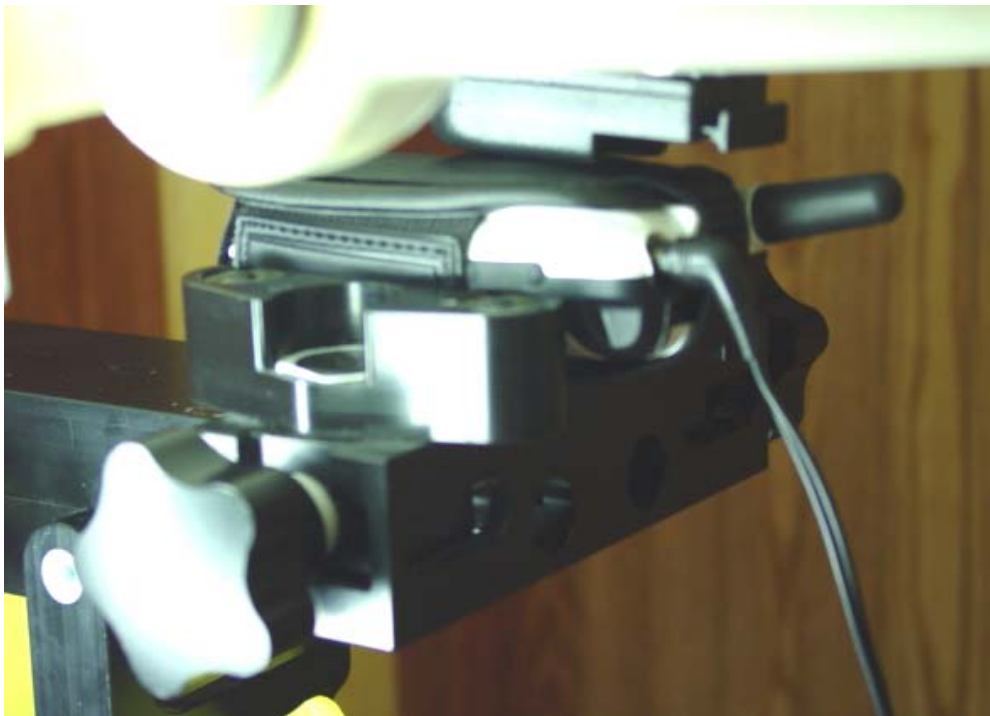
Figure 12.4 body SAR setup (with 22.5mm air separation)
