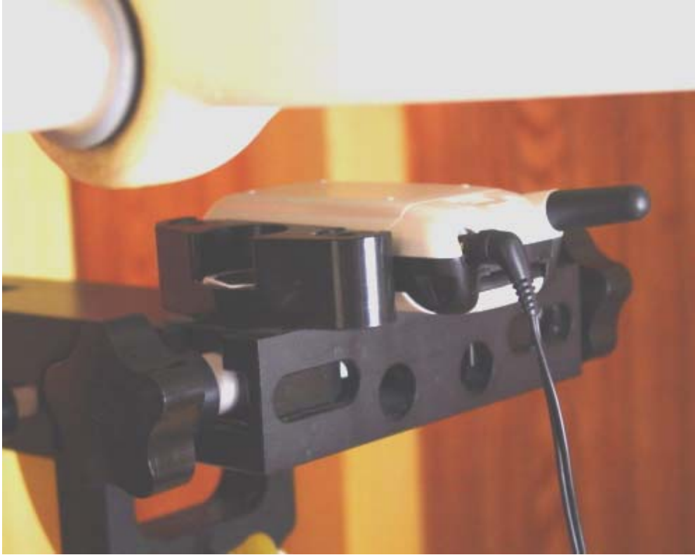
Figure 12.4 body SAR setup (with 22.5mm air separation)
