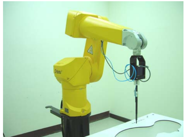
Fig. 5.2 Probe setup on robot
