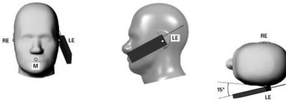
Figure 9.4 - Phone position 2, “tilted” position.
