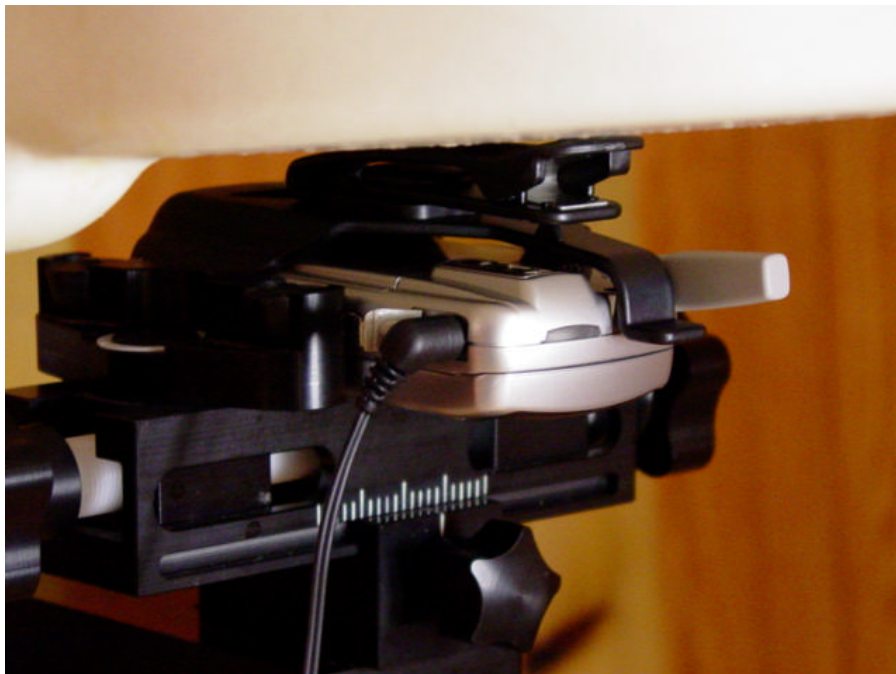
Figure 12.5 body SAR setup (with holster)
