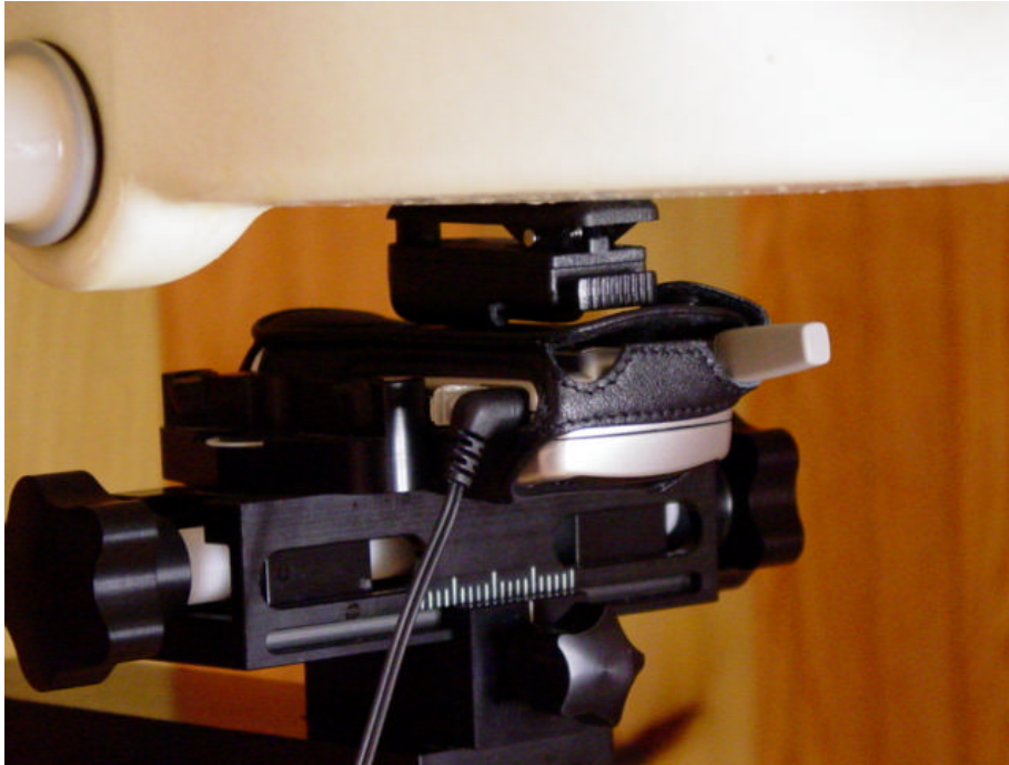
Figure 12.6 body SAR setup (with leather case)
