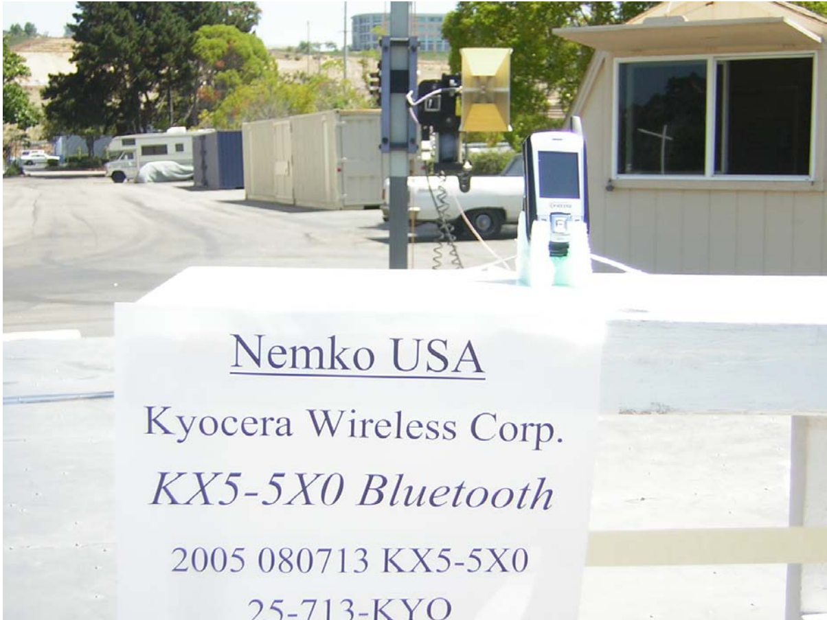
Photograph 6. Fundamental Radiated Emissions Test Configuration (Closed)
