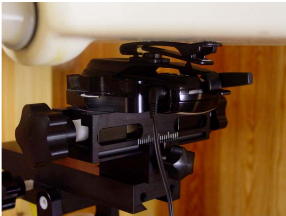
Figure 12.6 body SAR setup (with holster)
