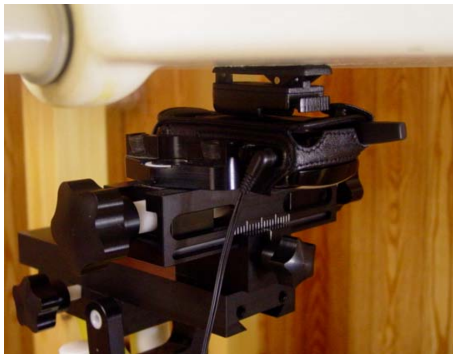
Figure 12.7 body SAR setup (with leather case)
