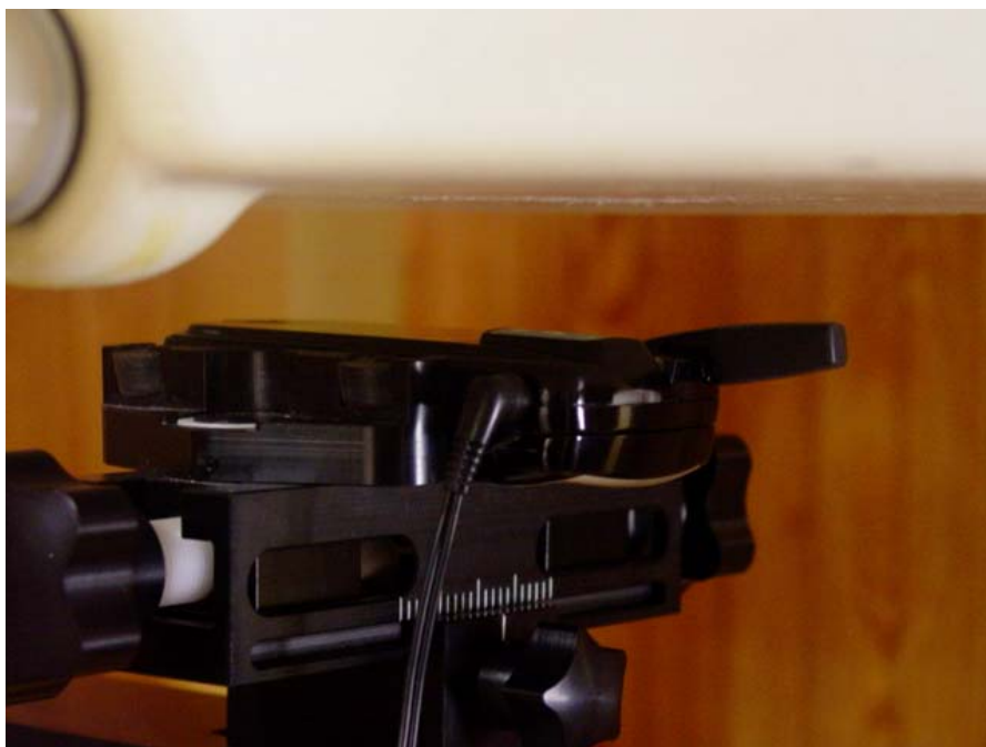
Figure 12.8 body SAR setup (with 25mm air separation)
